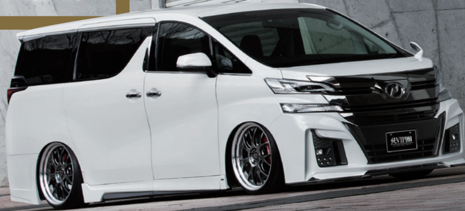
[30VELLFIRE] SIZE: [FRONT] : 21 X 10.0J INSET36(H)HYPER BLACK [REAR] : 21 X 10.0J INSET36(L)HYPER BLACK 20mm SPACER INSERT RIM DAGLIP STEP/RIM COLOR CUT ALUMITE
